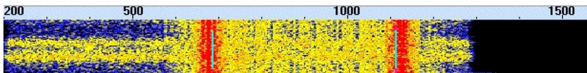
4. If you don't see the right peak, you may need to increase the frequency range of the RF spectrum/waterfall. On the right of the RF spectrum/waterfall click the 4.3 radio button in the Band KHz box.
