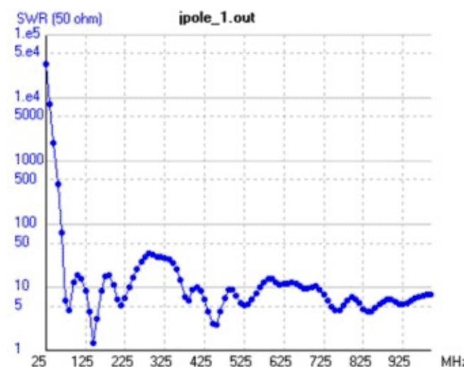
The J-pole antenna is named as such as it looks like the letter ‘J’. These antennas usually have good gain at their intended frequency. An advantage to J-poles is that their impedance can be matched to the coaxial cable easily by moving the connection points up and down. A J-pole can give 6.5 dBi gain or more.
